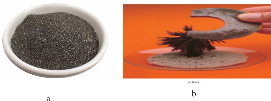
Figure 2.16 (a) the mixture contains iron filings and sand. (b) A magnet separates the iron filings from the mixtures.
