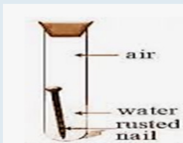
Figure: 2.15 rusting of iron
