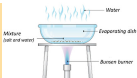
Figure 2.22: Evaporation of a solution
